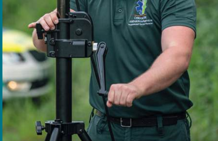
HAND WINCH TRIPOD WITH SAFETY LOCK
